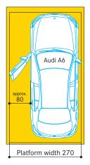
Depending on the vehicle model and the parking position of the vehicle on the platform, the space for opening the door varies. For comfortable conditions for getting in and out of the car, we recommend platform widths of at least 270 cm.
